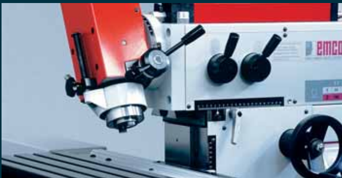
Vertical milling head. Vertical milling head with DIN 2080 SK 30 and clampable 45 mm quill travel. The vertical milling head swivels +/- 90°.
