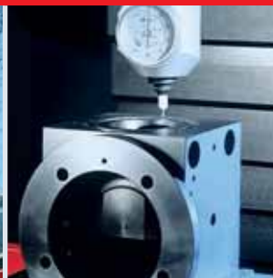
Setting up a part for milling with a 3D sensor
