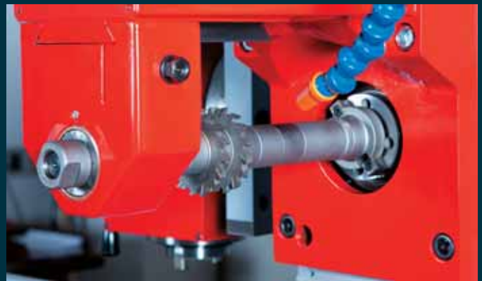
Horizontal milling. Horizontal milling with long milling arbor for clamping several milling tools. The overarm for supporting long milling arbors is mounted instead of the vertical milling head.
