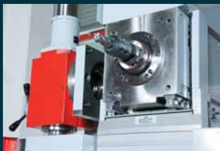
Changeover to horizontal milling. Horizontal milling spindle DIN 69871 SK 40
