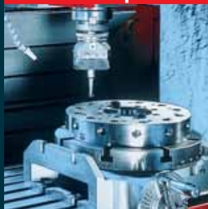
Machining a die-opener disc with the boring tool
