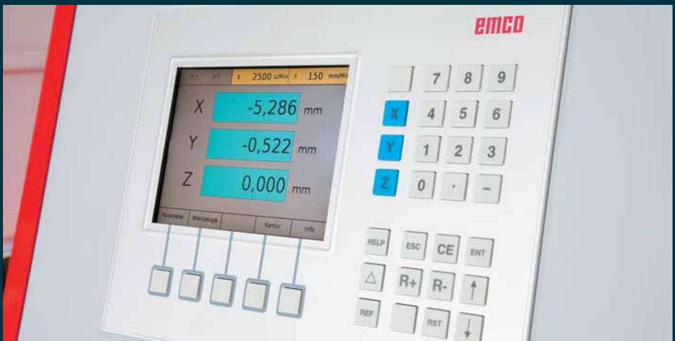
EMCO three axes position display for EMCOMAT FB-450 L and FB-600 L (standardly included)
