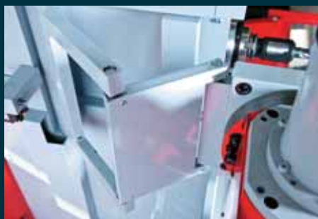
Swiveling device. Swivel-mounted vertical milling head. Controlled by end switch.
