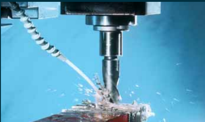
Vertical milling head. Drilling large diameters with the vertical milling head. Quill travel up to 80 mm.
