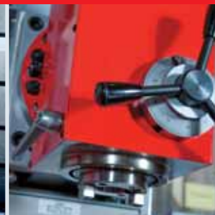
Vertical head with milling spindle DIN 69871 SK 40 with quill 80 mm
