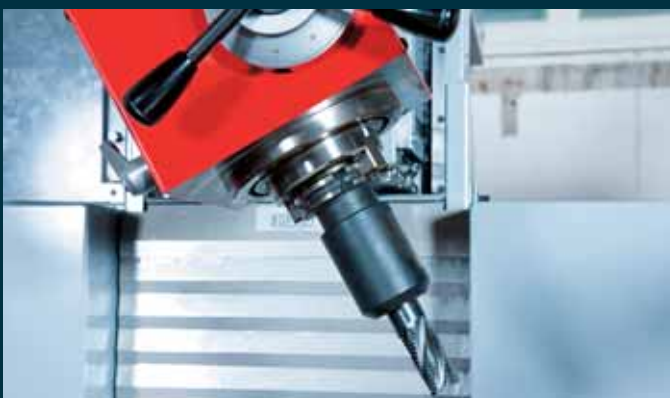
Swivel-mounted vertical milling head Swiveling the vertical milling head makes it possible to machine complex parts. +/- 90° swivel.
