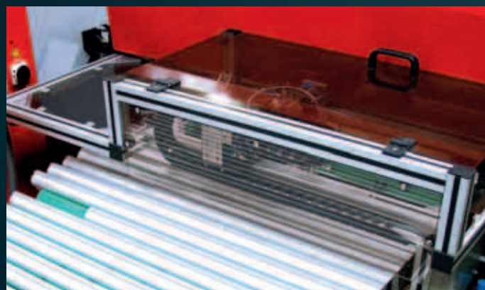
Infeed of profile bar stock using a chain feeding system (option)
